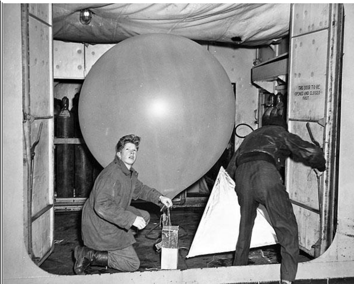
A weather balloon being inflated aboard ST. STEPHEN at Baker station. Also shown is the radiosonde and the radar reflector. Note the padded deckhead to ensure nothing can puncture the balloon. ( Photo believed to be taken by W.S. Walker via Sandy McClearn )
