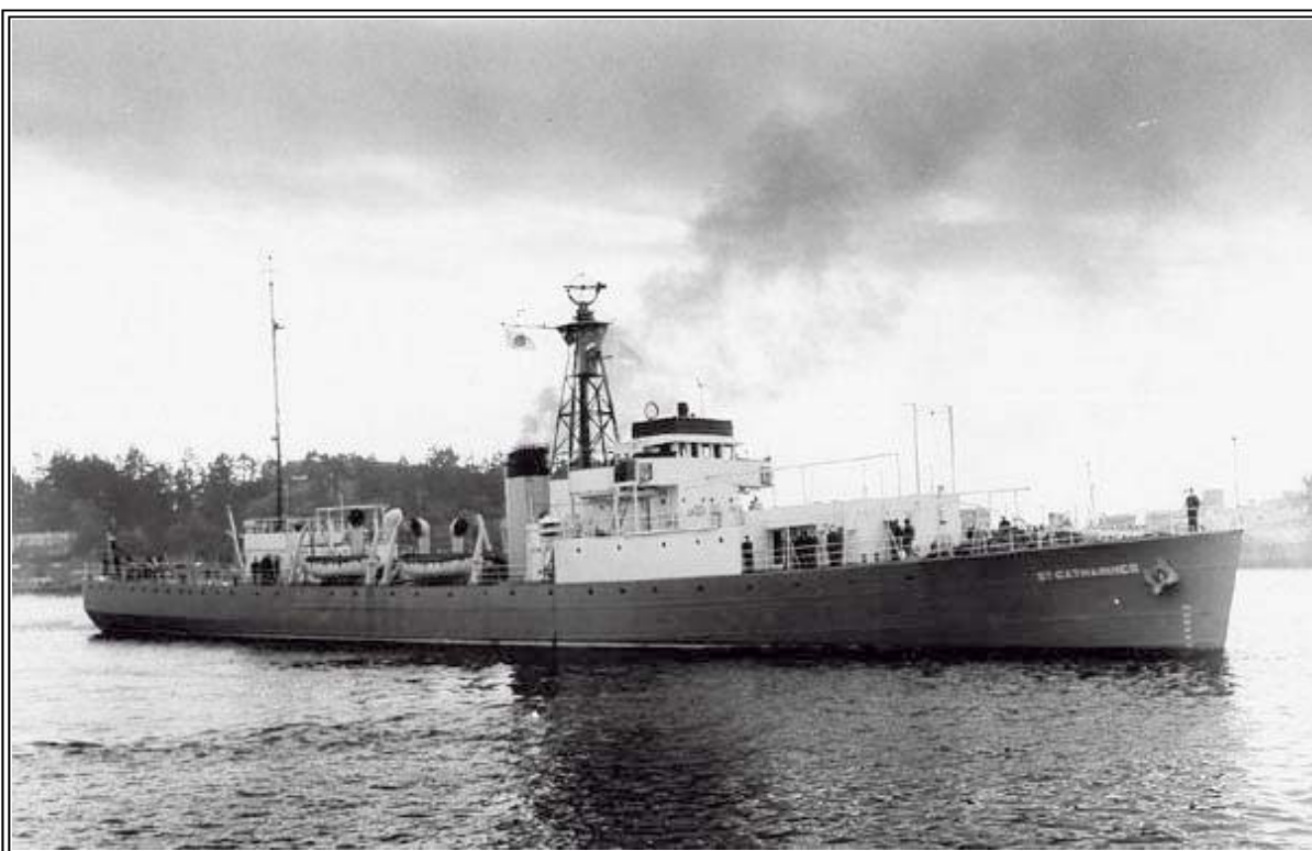
CCGS St.Catharines, call sign CGGQ. Her radar antenna is the 'AUK' type which means the ship is fitted with the 277P radar. Note the flush deck and modernized bridge. It's estimated that this photo was taken between 1962 and 1967. (Canadian Coast Guard photograph submitted by Spud Roscoe)
