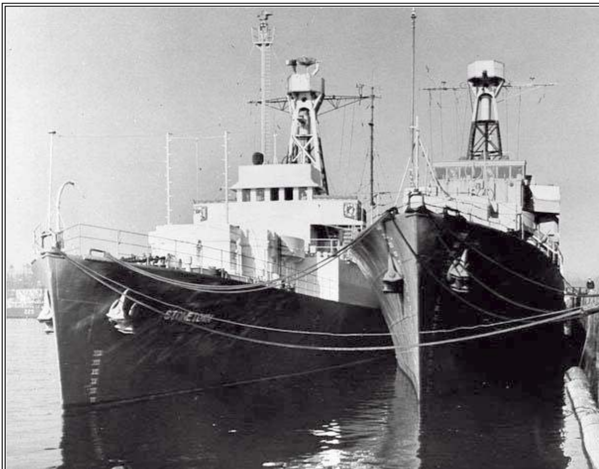
CCGS Stone Town outboard of CCGS St. Stephen. Stone Town is fitted with her 277P radar as attested by aerial outfit 'AUK'. Because St. Stephen had become a parts source to support the other two ships still in service, she never left port. Notice the missing 277 antenna on her foremast when compared to Stone Town. ( Canadian Coast Guard photograph submitted by Spud Roscoe VE1BC )
