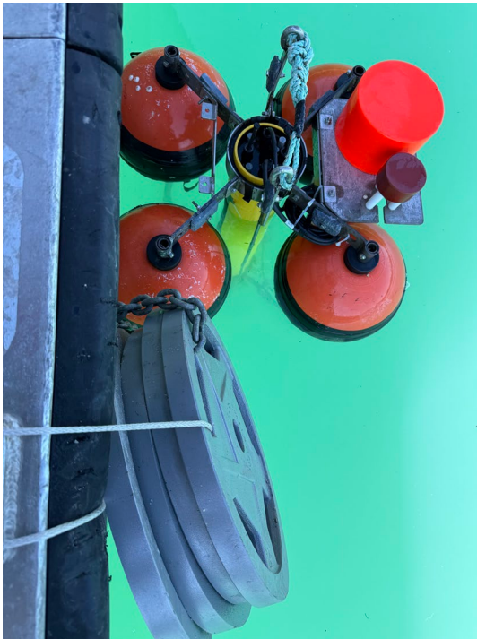
Figure 2: Deployment of Acoustic Mooring from R/V Doug Anderson.
