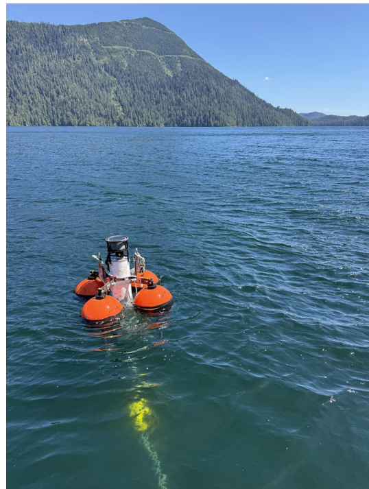
Figure 2: Deployment of Acoustic Mooring from R/V Doug Anderson.
