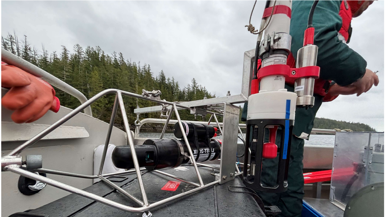
Figure 2. RBR CTD integrated with LIIST instrument
