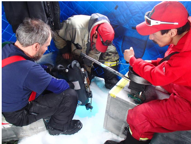
Mike Dempsey, Ryan Green and Johnny Ruben in a tent lowering a Niskin sampler through sea-ice
