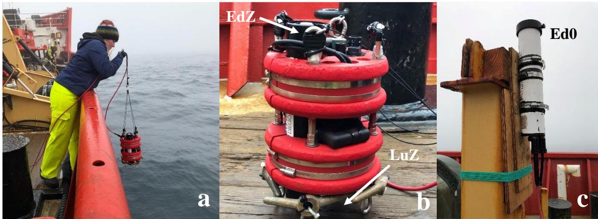
**Fig 4.** Setup of the C-OPS system, showing (a) a typical deployment off the bow and the three radiometers that simultaneously collect data: (b) the EdZ profiling radiometer measuring downwelling radiance and the LuZ profiling radiometer measuring upwelling radiance, as well as (c) the Ed0/surface reference radiometer.
