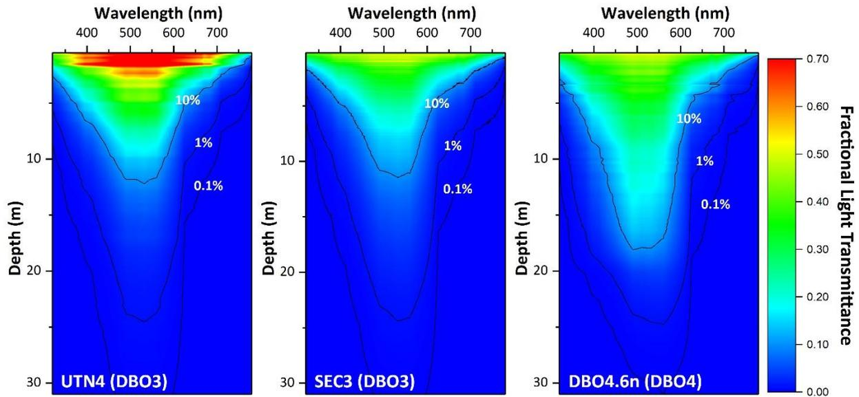
**Fig 5.** Example optical profile data from the C-OPS instrument for stations UTN4, SEC3, and DBO4.6n collected in July 2018.
