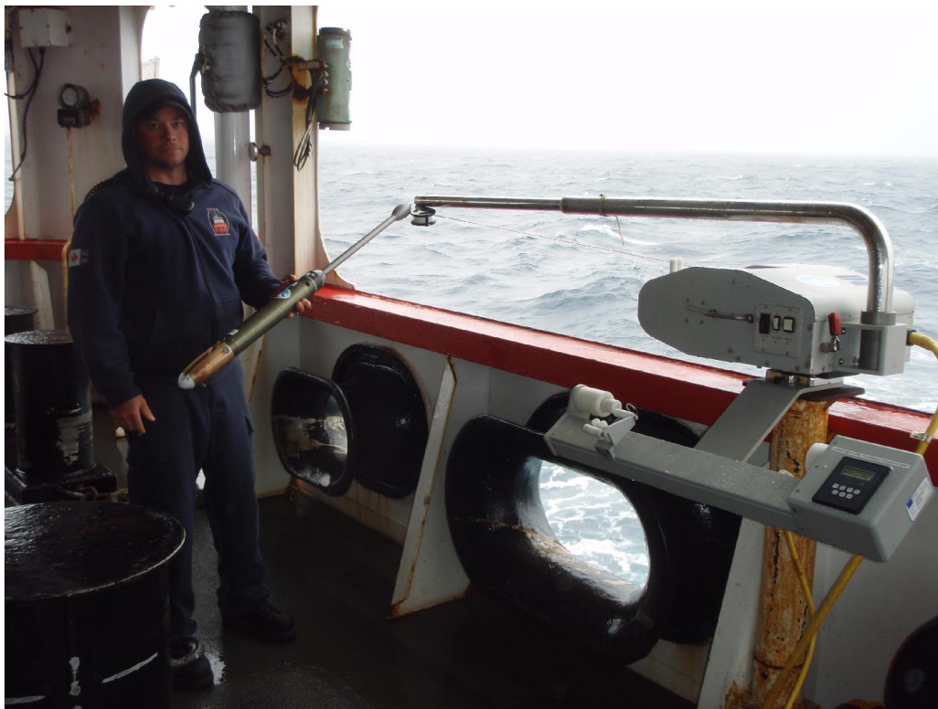
Figure 3. Underway system used to deploy Conductivity, Temperature, Depth probe to 400 m every 6 hours while crossing NE Pacific.
