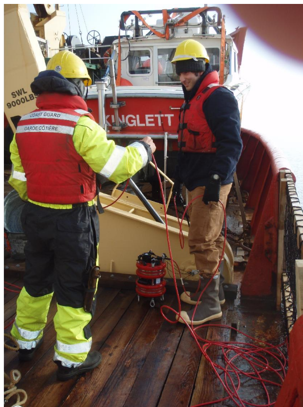
Figure 10. Apparent optical property package (C-OPS) that was lowered over the side of the ship.
