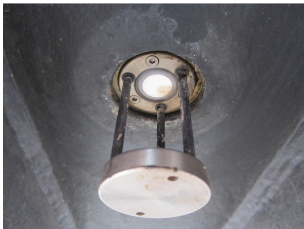
Figure 24: View of the Valeport MiniSVS probe as it extends out of the hull.
