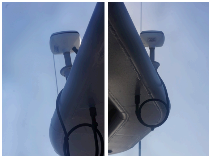
Figure 5 Left, bridge navigation antennas mounted on the flying bridge bimini frame looking aft, starboard and port, respectively.
