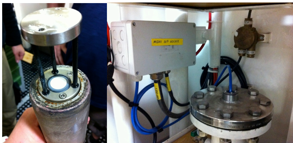
Figure 23: Left, Valeport MiniSVS probe. Right, SVP secured in its tube.
