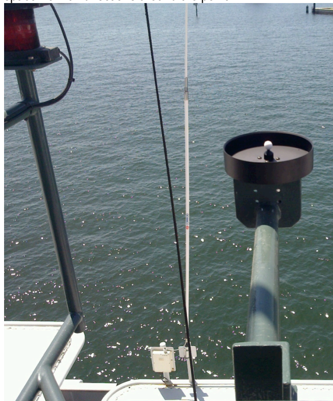
Figure 14: Biospherical Surface sensors, mounted on arms extending from the lower radar platform.
