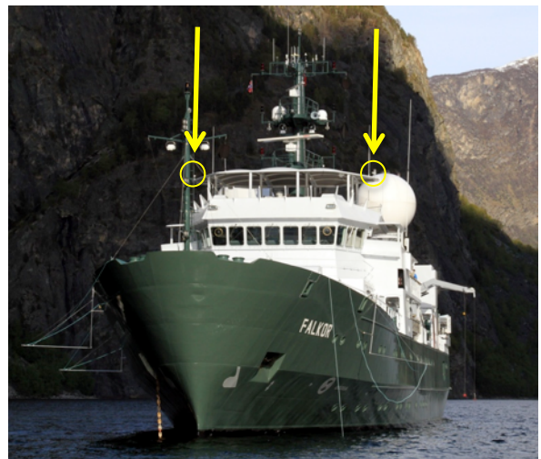
Figure 5 Left, bridge navigation antennas mounted on the flying bridge bimini frame looking aft, starboard and port, respectively.
