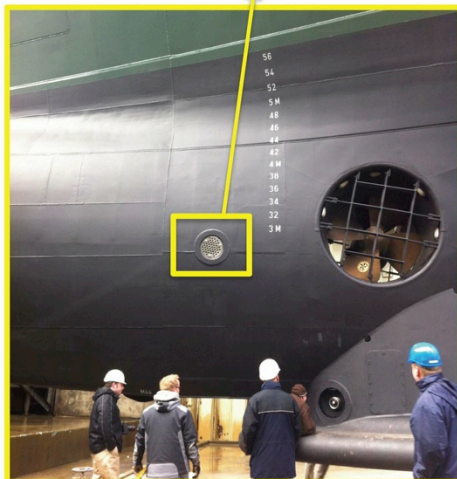
Figure 16: Position of the scientific seawater system intake, just forward the bow thruster on the port side.
