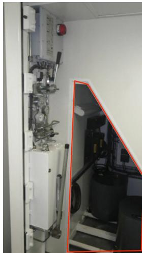
Figures 10 & 11: View of the Seapath MRU mounted on the bulkhead after the door is removed.
