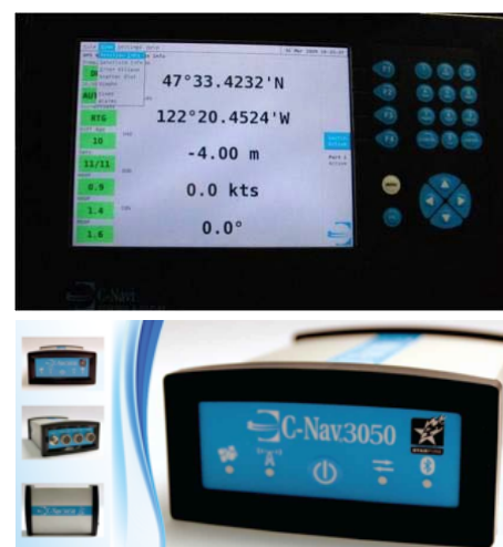
Figure 8: C-Navigator II display with CNAV 3050 receiver.
