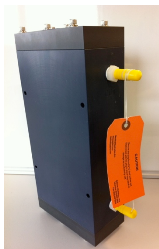
Figure 22: SBE 45 Micro Thermosalinograph.
