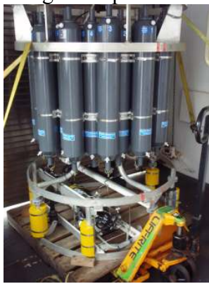
Figure 6. The 24 Niskin-bottles rosette system successfully used during the trip to collect water at selected depths.
