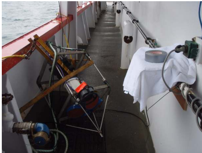
Figure 8. The 150 kHz Acoustic Doppler Current Profiler (ADCP) and the 4-frequency Acoustic Zooplankton and Fish Profiler (AZFP) in their stainless steel frame on deck just prior to deployment.
