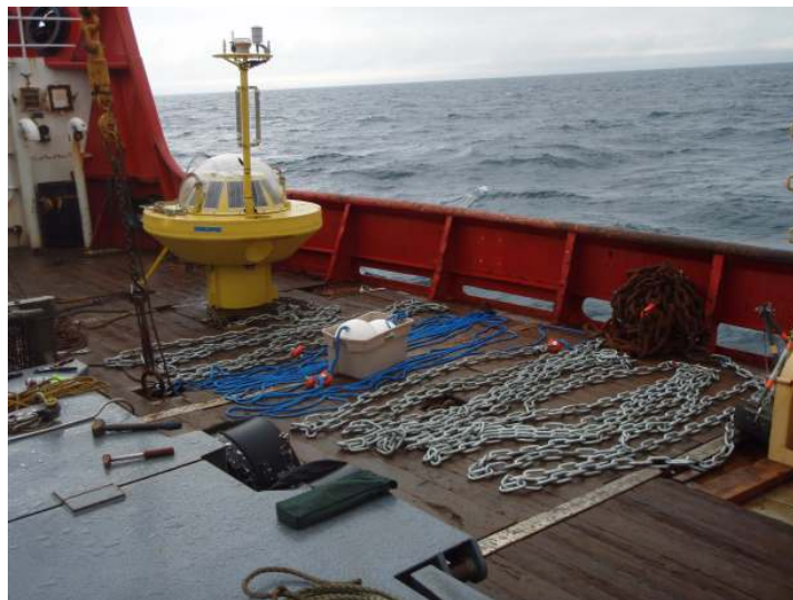
Figure 1. Axys wave buoy shortly before deployment near the Bering Strait ( 65^{\circ} 00.574'N 169^{\circ} 27.211'W ).
