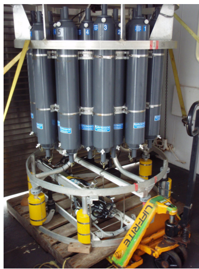
Figure 12. The 24 Niskin-bottles rosette system successfully used during the trip to collect water at selected depths.
