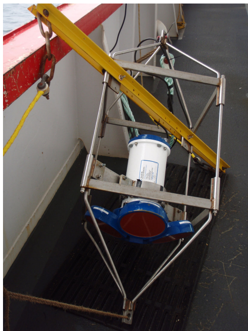
Figure 9. The 150 kHz Acoustic Doppler Current Profiler (ADCP) in its stainless steel frame on deck just prior to deployment.
