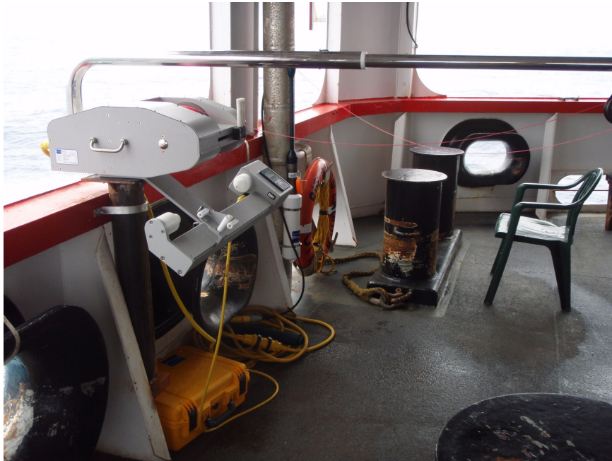
Figure 6. Underway CTD system mounted at the stern of the ship. During the trip profiles were obtained at least every 6 hours across the NE Pacific to a maximum depth of 400 m. A total of 46 profiles were collected during the cruise.
