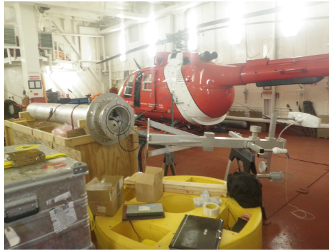
Figure 2: Assembled mast minus the scan head for the UV/Vis spectrometer and wind sensor.
