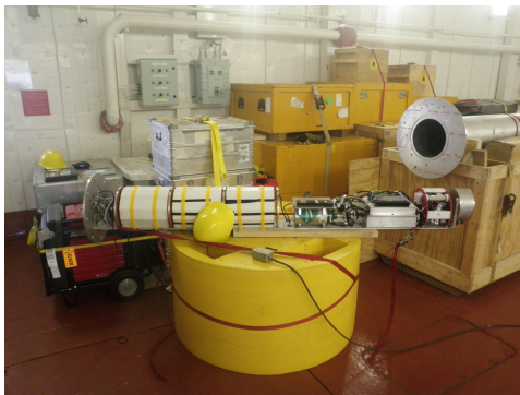
Figure 1: The instrumentation for the O-buoy. Starting from the left of the picture the tray holds: 3 Li battery packs for power during winter months when the solar array does not work, CO 2 tanks used as standards for the CO 2 sensor, the ozone detector and supervisory computer which controls buoy operations, the CO 2 sensor, and finally the spectrometer for the differential optical absorption spectroscopy done by the buoy to detect BrO
