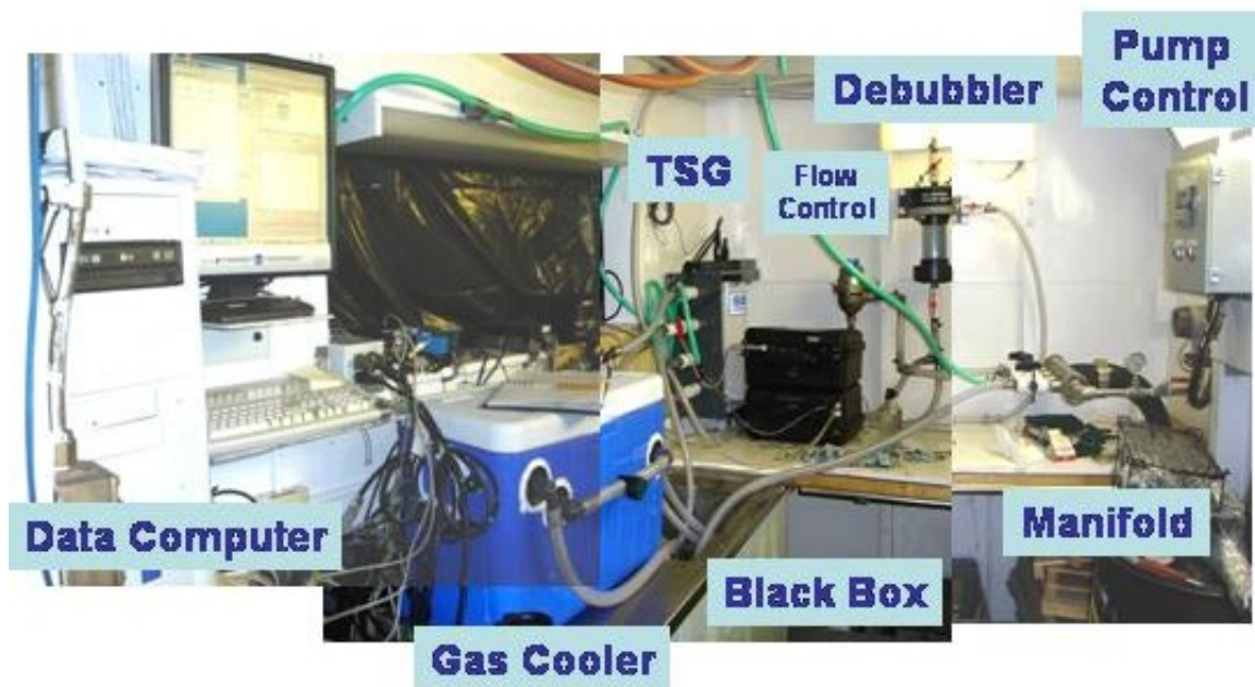
Figure 29. Seawater loop system providing uncontaminated seawater from 9m depth to the science lab for underway measurements
