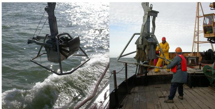
**Figure 1 Launching and retrieval of the box corer.**
