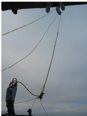
**Figure 3.** Camera with cable running through cable feed wheel (attached to encoder for line out)
