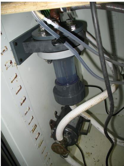
Figure 3: Sea-water reservoir, aka, "the bucket of doom" showing sump pump.
