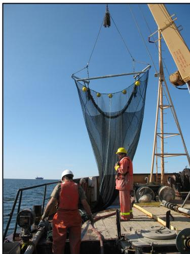
The mouth of the beam trawl measured 3m x 3m, and the net was 9.4m in length. The main body of the net was composed of 3.75cm stretched mesh, with a 1.25cm stretched mesh liner on the inside of the bottom panel. The cod-end was lined on the outside with 0.3cm square mesh.
