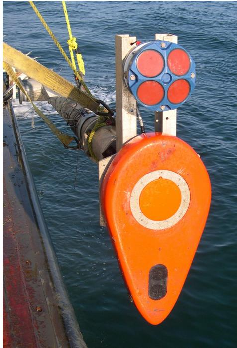
**The ADCP mounted forward of the acoustic pod on the acoustic arm.**
