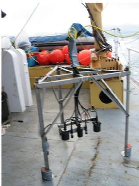
**Figure 1.** Camera, lasers, lights and depth transducer attached to tripod frame with weights.
