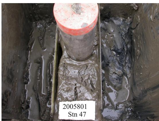
**Figure 2 Push core taken in box core**
