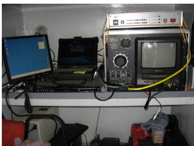
**Figure 4.** Camera console/viewing area, laptop and recording unit within housing unit.
