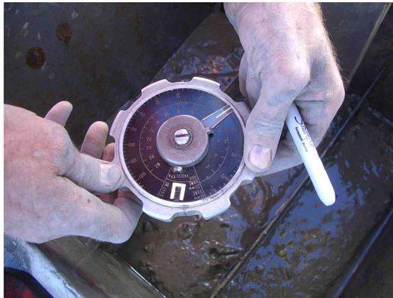
**Figure 4 Field hand vane undrained shear strength measurements on sediments retrieved with the box corer.**
