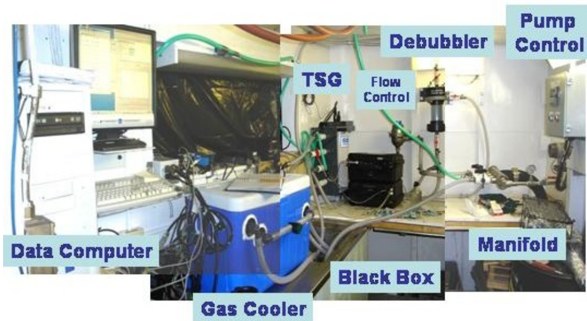
Figure 13. Seawater loop system providing uncontaminated seawater from 9m depth to the science lab for underway measurements.
