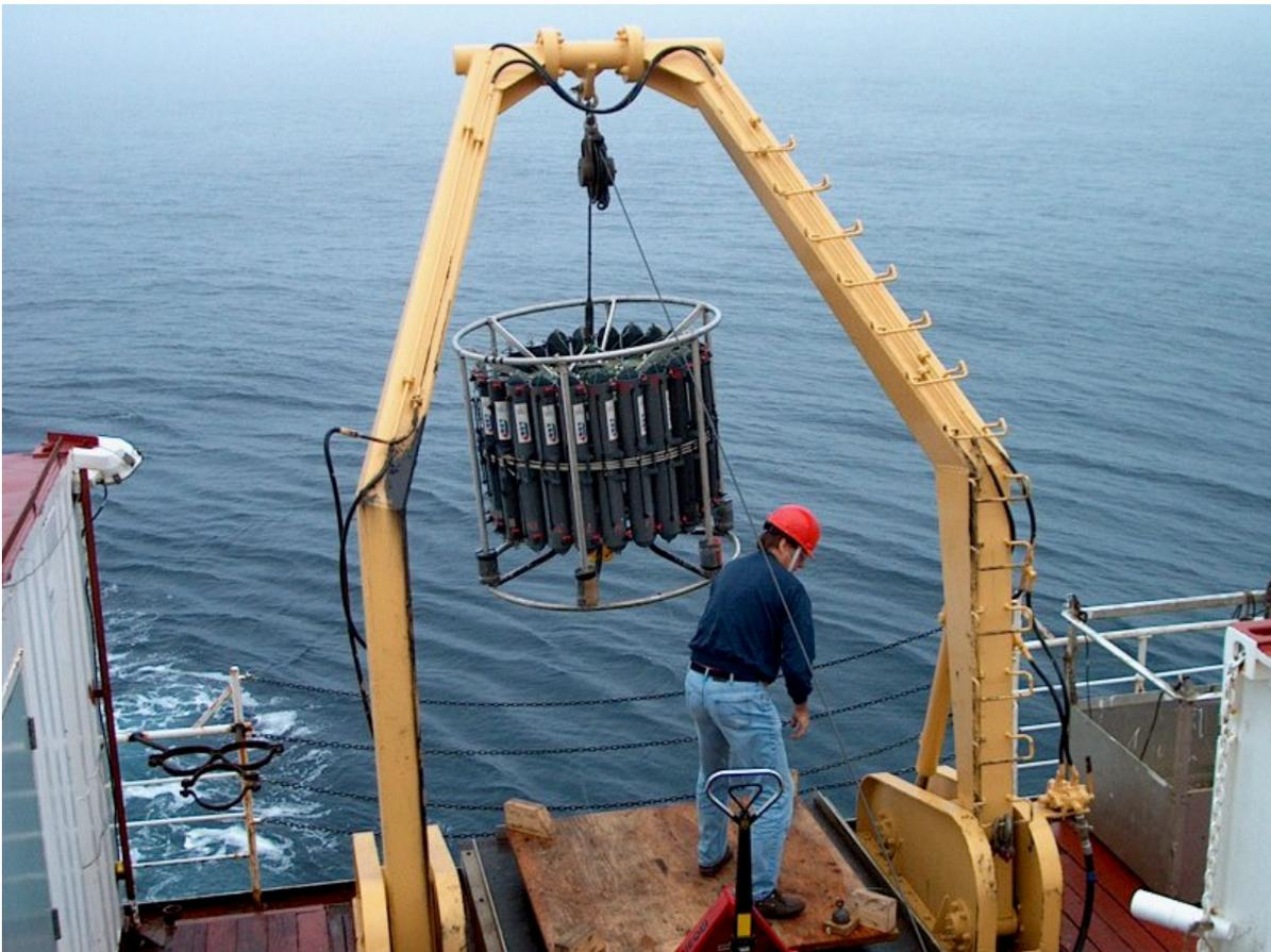
Before each cast, when approaching the location of a science station, the Rosette was prepared for launching by emptying all sampling bottles, hooking the lanyards from the top and bottom flaps of each bottle into the Carousel pylon, and closing the valves and vents on the bottles. The station name and location, cast particulars, sounding and information about sea state were entered in the CTD log book, as well as any other factors that might affect or alter how the system behaved.
