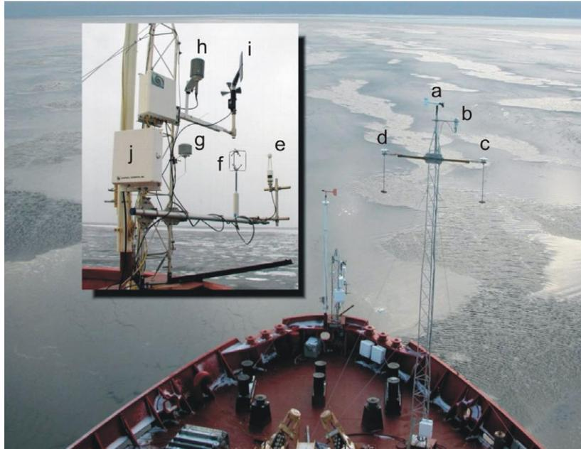
**Figure 6** The foredeck of the Pierre Radisson equipped with a 10 m (nominal) meteorological tower and a 2 m (nominal) tower at the bow of the ship that was used for flux measurements (in medallion). See table 1 for details on sensors.
