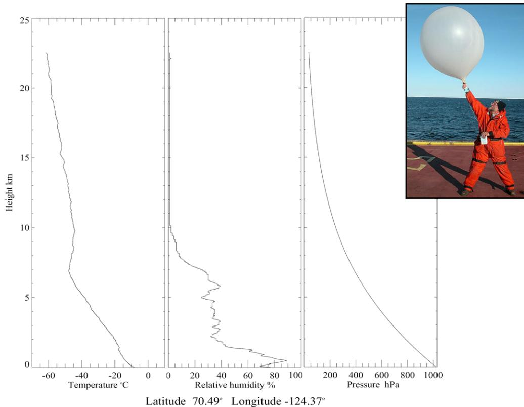
**Figure 8.** An example of a radiosonde profile, showing atmospheric temperature, humidity and pressure as a function of height. (13 October 2002, 11:52 GMT)
