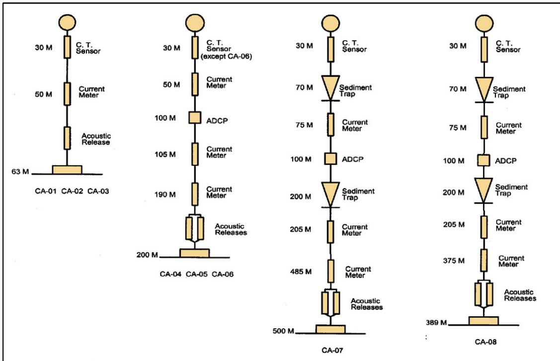
**Figure 4.** Schematic representation of the 8 CASES moorings deployed from the CCGS Sir Wilfrid Laurier from 12 September to 19 September 2002 (courtesy of Ingram, Carmack, van Hardenberg).
