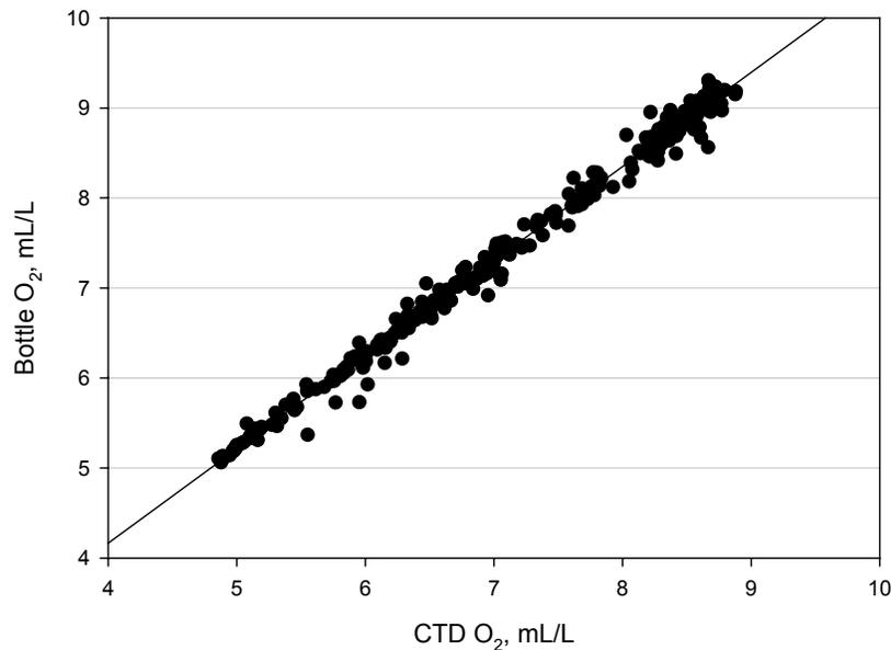
**Figure 5.** Correlation between dissolved oxygen ( $O_2$ ) determined by colorimetric Winkler titration and Seabird  $O_2$  sensor. Slope: 1.05;  $r^2 = 0.993$ . (Preliminary data: Lisa Miller)
