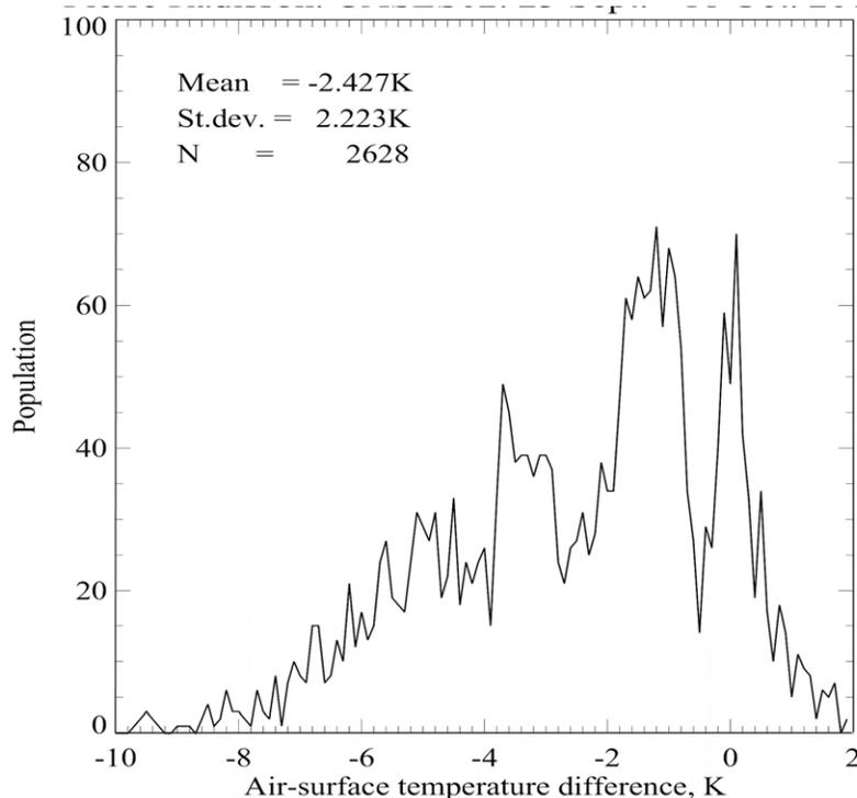
**Figure 7.** Histogram of the air-surface temperature difference measured by the M-AERI between 23 September and 18 October 2002.
