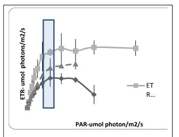
Figure 1. Representative PvsE curves: shelf slope (Feb 1), pelagic (Station Papa 50 N, 145 W, Feb 9) and coastal (Hecate Straight, Feb 14). Shown are mean electron transport rates (+/- SD, N= 3-5) as derived from PAM fluorometry over increasing PAR levels. The blue band denotes the approximate light saturation level for photosynthesis.
