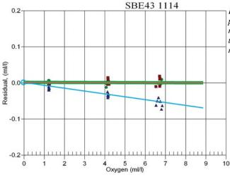
**Figure 2.** SBE 43 sensor SN 1114 original factory calibration (green dots); post-recovery calibration prior to sensor cleaning (blue triangles); re-calibration after sensor cleaning (red squares). Note the loss of sensitivity in the post-recovery calibration (blue triangles) is strictly linear, and that cleaning restored the SBE 43 to its pre-deployment calibration accuracy (red squares).
